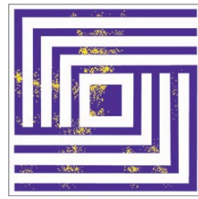
Atypical failure: Possible cause Poor quality "wet steam"
